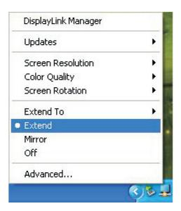
Mirror: This option allows you to set the DisplayLink Manager to Mirror mode. Enabling this will let you see an identical desktop image on the additional monitor.
